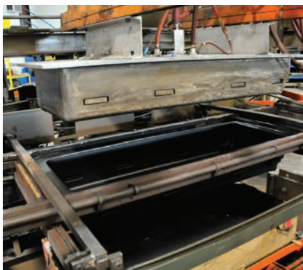
Vacuum mold for keyboard case
