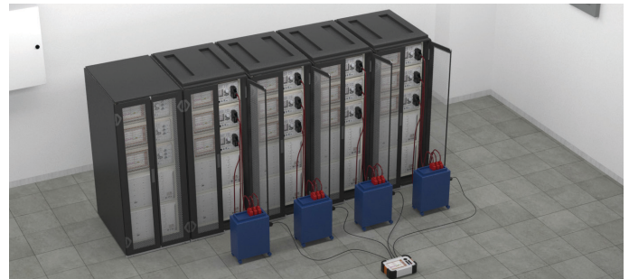
Transmitter and receiver tests for mobile-radio base stations
