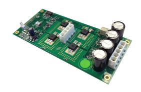
Thermoelectric Temperature Controller TEC24VCNTLRN, TEC48VCNTLRN Models
